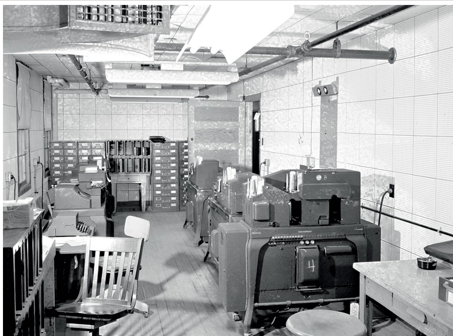
Fig. 1 | IBM punch-card accounting machines used at Los Alamos during the Manhattan Project. At the back there are the IBM 601 multipliers with and without divide units, at the front there is the duplicating keypunch. The photograph was taken some time after November 1944. Image courtesy of Los Alamos National Laboratory.
